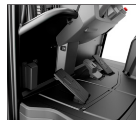
Dual pedal system - forward and reverse.
