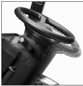
Responsive hydrostatic steering
