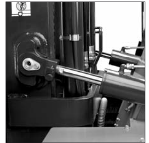
Sealed tilt cylinders
